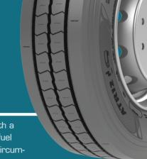
Next generation trailer tire for regional applications designed with a wide tread to reduce irregular wear, a tread compound to offer better fuel efficiency, solid shoulder ribs that improve wet braking, and innovative circumferential grooves for quicker water evacuation.
