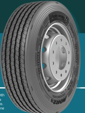
An All Position tire for long-haul and regional applications with a five-rib pattern to maximize surface contact and bear load evenly, and a wider, unique tread pattern to prevent irregular wear and enhance tire life. Center rib sipes enhance braking and steering in wet conditions, and stone ejectors on every groove ensure better traction and grip.
