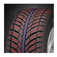
A FUSION OF SIPES. Summer and winter sipes lead to effective dry braking and greater traction in snow.
