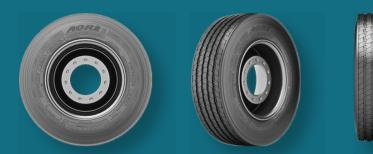
An All Position tire for long-haul and regional applications with a five-rib pattern to maximize surface contact and bear load evenly, and a wider, unique tread pattern to prevent irregular wear and enhance tire life. Center rib sipes enhance braking and steering in wet conditions, and stone ejectors on every groove ensure better traction and grip.
