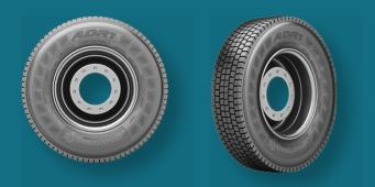
A drive axle tire for regional applications with an open shoulder design that provides quicker water evacuation and superior road grip, deeper grooves for better traction and prolonged tire life, and optimized block shape and unique tread design to prevent irregular wear and stone retention.
